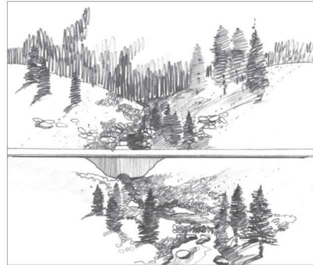
*A | Seasonal and ephemeral stream courses can be placed in a culvert for short sections as they cross the corridor. Naturalized channels should be maintained and enhanced on both the uphill and downhill sections as a landscape and visual feature.*
